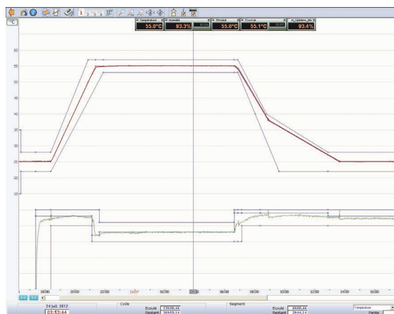
Example of an IEC 60068-2-30 test
